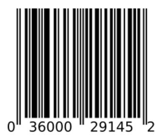
What do the numbers mean? The first digit denotes the encoding systemed used, the next 5 digits typically denote the manufacturer code and the 5 digits after that typically denote the product code. The last digit is the check digit which can detect if an error is present in the code. Assuming the digits are labelled  $a_1, \ldots, a_{12}$  they must satisfy the *check digit equation*
